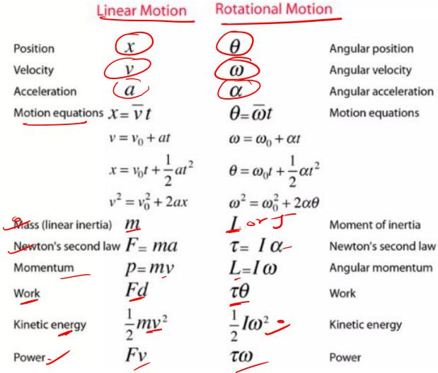
Angular position Angular velocity Angular acceleration Motion equations
